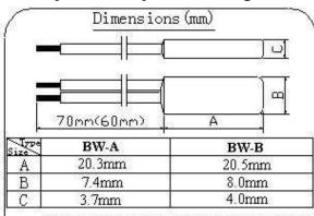
Notes: The lead wire can be made according to the customers' requirements. The above dimension is the one non-insulated sleeving.
